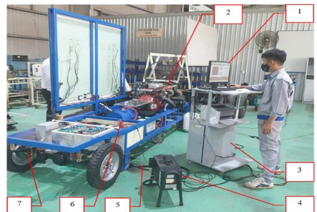
Figure 14. Experimental setup for measuring diesel engine emissions 1- Computer; 2- Diesel engine; 3- CPU; 4- HESHBON HD-410 emission meter; 5- Probe; 6- Battery clamp; 7- Speed sensor
