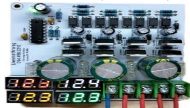
Figure 9. Active Battery Balancing Circuit 48V/Max 20A on HEV model
