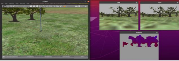
Figure 3. Stereo camera simulation in Gazebo with an obstacle
