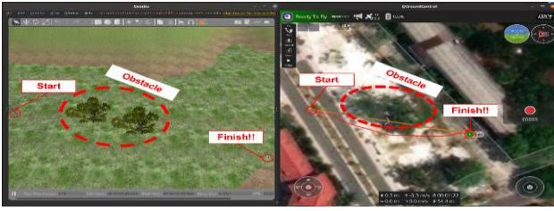
Figure 7. The flight path of UAV from Start point to Finish point in an environment with obstacles
