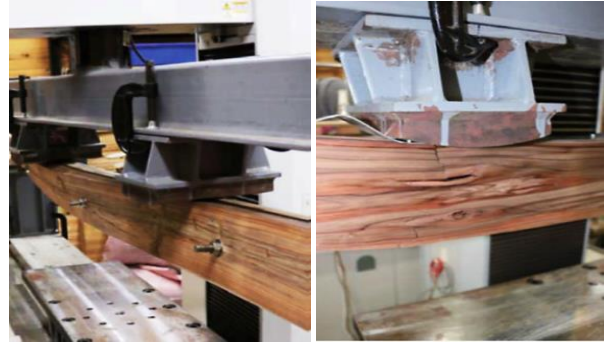
Figure 4. Cracking in timber lower chord of Type F beam (left) and type D (right)
