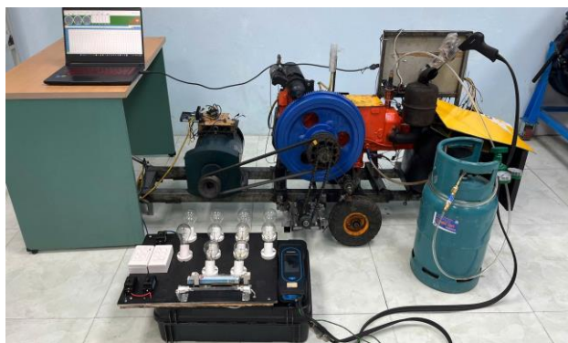
Figure 16. Layout of the dual fuel engine using flexible syngas-biogas-hydrogen fuel in the experimental system
