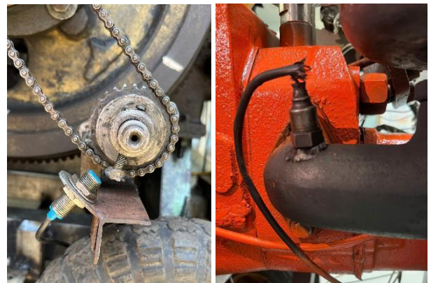
Figure 15. Arrangement of the TDC sensor (a) and the lambda sensor (b)
