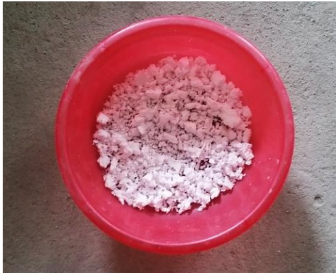
Figure 1. RPS used for making concrete
