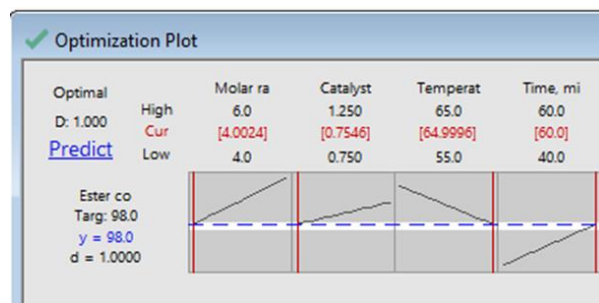
Figure 5. Optimal condition of process factors for biodiesel production
