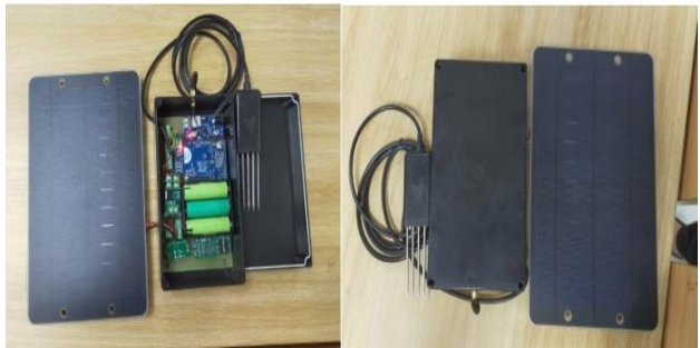
Figure 2. Soil quality measurement node
