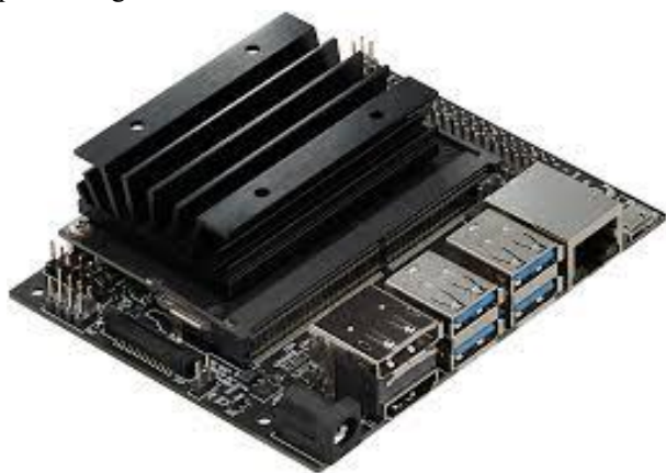
Figure 2. The edge device, NVIDIA Jetson Nano Developer Kit B01, used in the experiments
