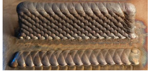
a) Sinusoidal zigzag thin-walled structure
