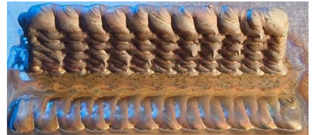
c) Square-angled zigzag thin-walled structure
