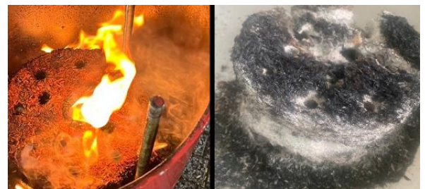
Figure 14. RDF rice husk pellets during combustion (a) and after combustion (b)
