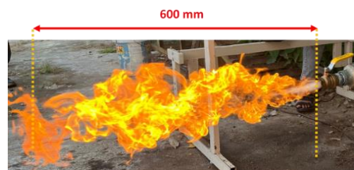
Figure 8. Figure depicting the syngas flame combustion at the gasifier outlet
