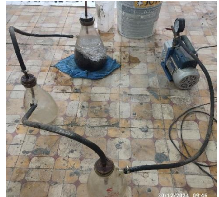
Figure 4. Test of maximum specific gravity and density of loose bituminous paving mixtures
