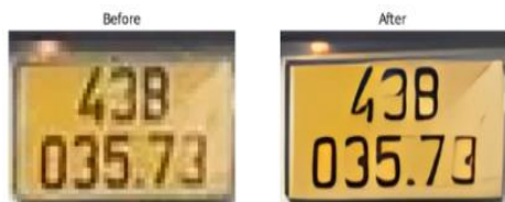
Figure 11. License plate preprocessing results after passing through Real-ESRGAN
