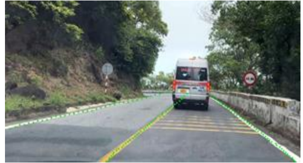
Figure 6. Lane detection results of the UFLDv2 model on real-world images
