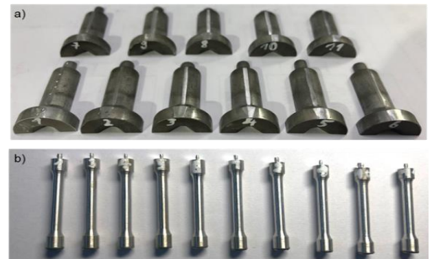
Figure 8. Specimens for microhardness and tensile testing after T6 heat treatment
