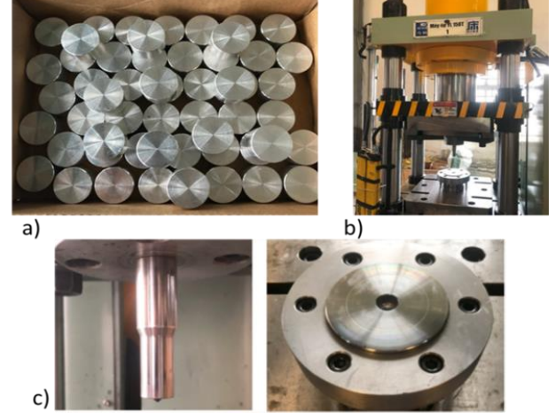
Figure 2. Initial billet (a), hydraulic press (b), and forward extrusion die (c)
