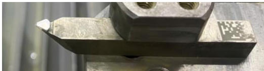
Figure 4. Diamond turning tool
