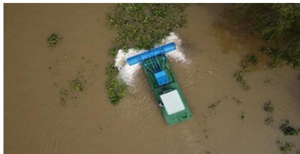
Figure 1. The MPLB-01 water hyacinth shredding machine under actual operating conditions
