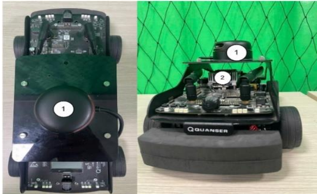
Figure 1. Experimental platform: (1) RPLIDAR A2, (2) NVIDIA Jetson TX2
