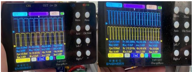
Figures 11. Encoder signals at SET = 40: (a) without Kalman filtering, (b) with Kalman filtering
