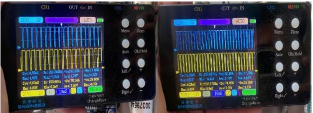
Figures 12. Encoder signals at SET = 70: (a) without Kalman filtering, (b) with Kalman filtering
