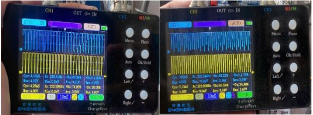
Figures 13. Encoder signals at SET = 110: (a) without Kalman filtering, (b) with Kalman filtering
