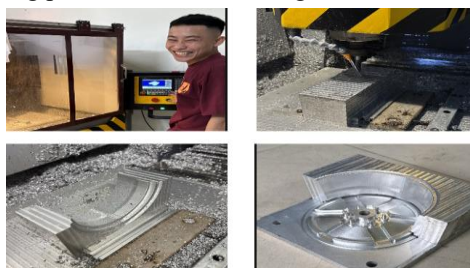
Figure 27. Machining of mold cage structures
