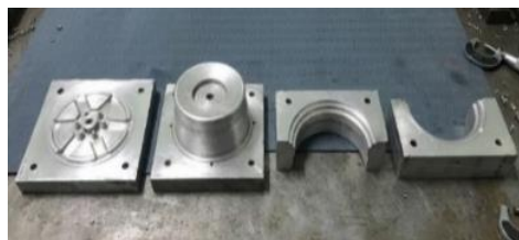
Figure 28. Mold cavities for automobile wheel casting after complete CNC machining
