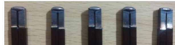
Figure 5. Surface photographs of the welds on copper hairpin samples after blue laser welding using the Spiral–Elliptical trajectory
