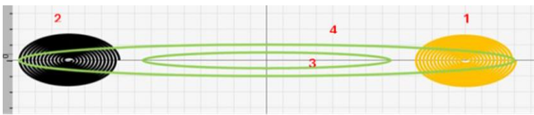
Figure 2. Spiral–Elliptical scanning trajectory: (1) Spiral 1, (2) Spiral 2, (3) Elliptical 3, (4) Elliptical 4
