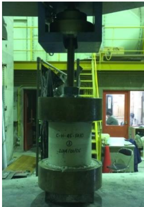
Figure 2. Direct tensile strength test
