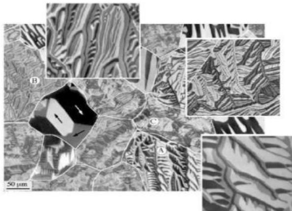
Figure 1. Magnetic domains of FeSi alloy is thick of 0.5 mm
