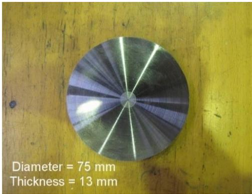
Figure 4. Workpiece Dimensions
