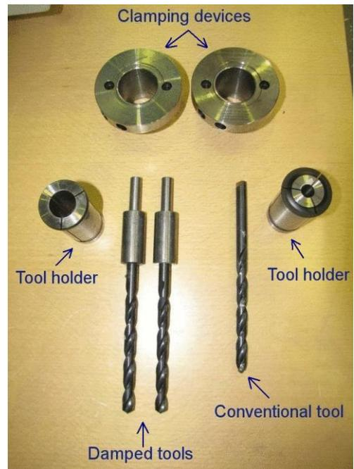
**Figure 3.** Tools and Clamping Devices
