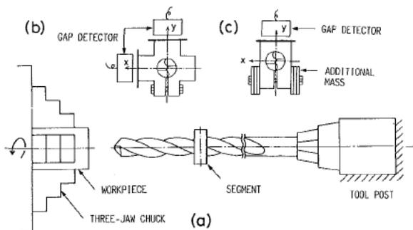
Figure 1. S. Ema Long Drill Operation Experiment
