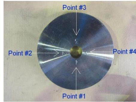
Figure 7. Surface Roughness Measured Points
