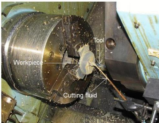
Figure 5. Machining Test in the Lathe Machine
