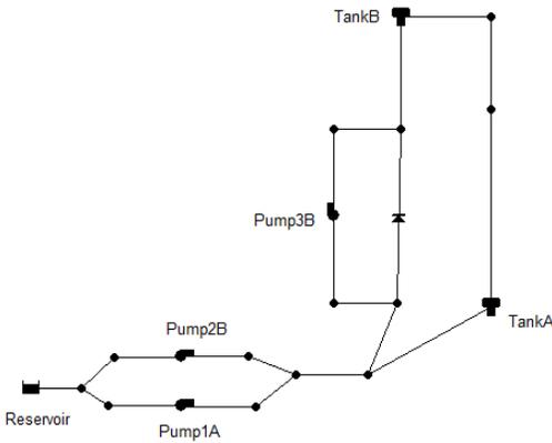
Figure 2. VanZyl water distribution network [9]
