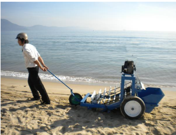
Figure 7. Rubbish collecting by man-pulled beach cleaning machine
