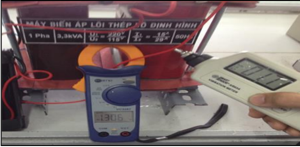
Figure 14. Results of the effective-vibration level in case the magnetic leg and yoke have not been fixed.
