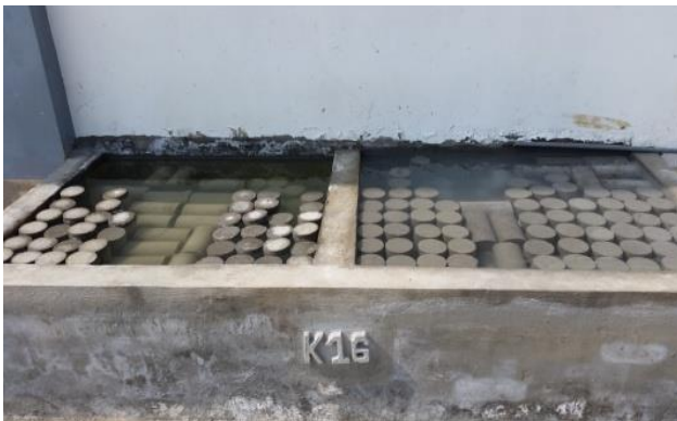
Figure 1. Concrete specimens were cured in water
