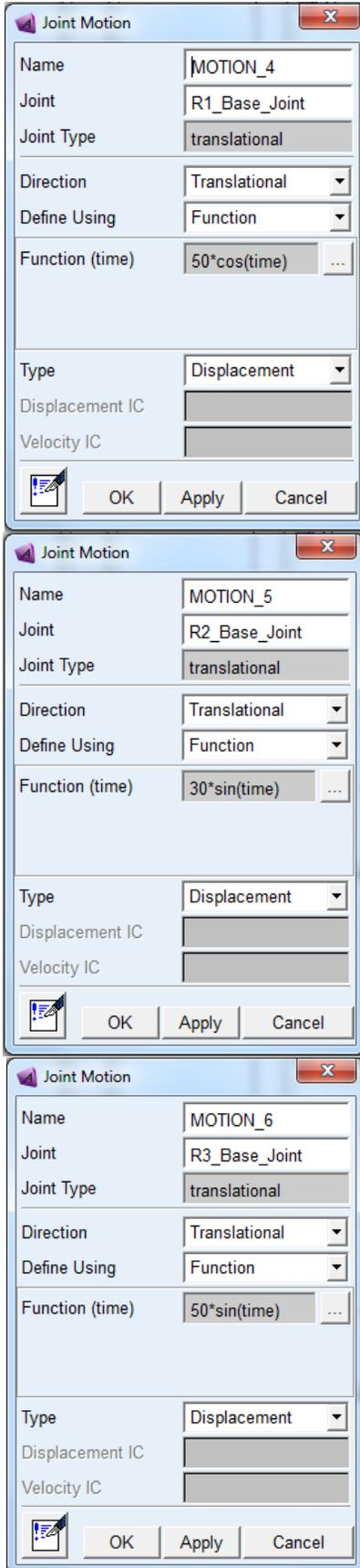
Figure 5. User windows of actuator motion
