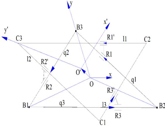
**Figure 2.** Kinematic structure of the planar manipulator
