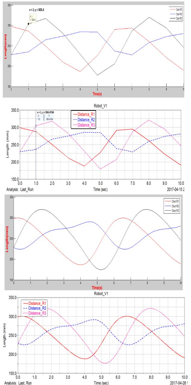
*Figure 4. Comparison of position of the actuated joint q<sub>1</sub>, q<sub>2</sub>, q<sub>3</sub> between result derived from Matlab and Adams view with step period = 0.1 s*
