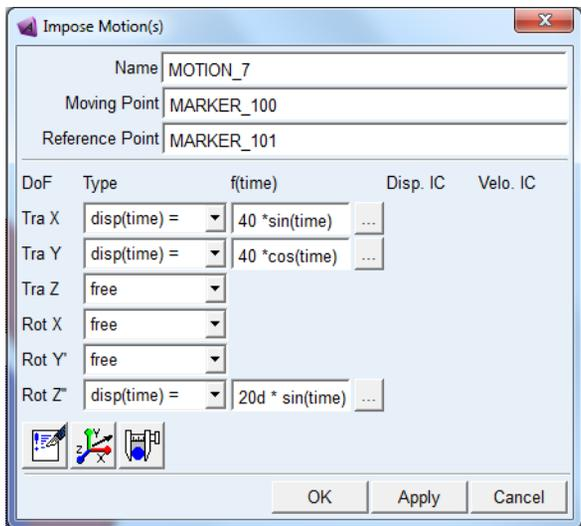
*Figure 3. User windows of general motion of the moving platform*
