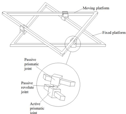
Figure 1. Triangular planar manipulator
