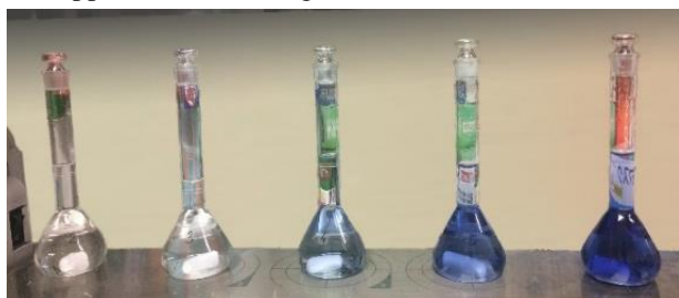
Figure 1. Samples of phosphorus standard solution (Phosphorus concentration 0.02; 0.2; 0.5 and 1.0 ppm)
