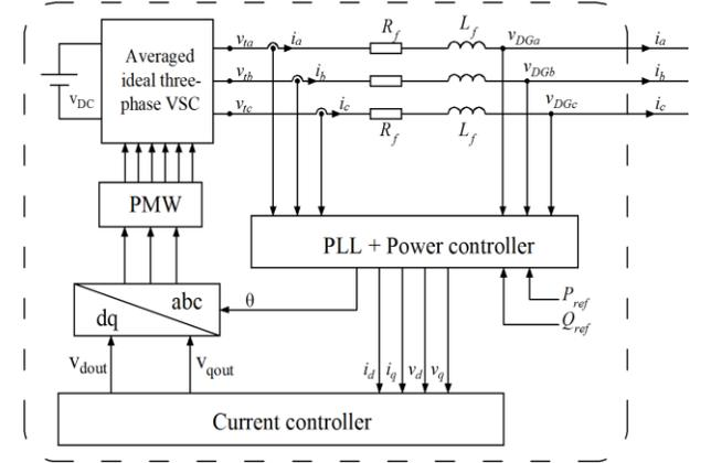
Figure 2. The overall control diagram of VSI
