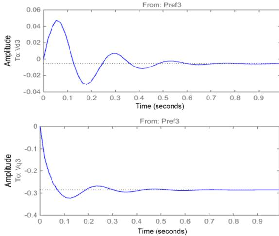
Figure 11. Response voltage  $V_{dq3}$  from  $P_{ref3}$
