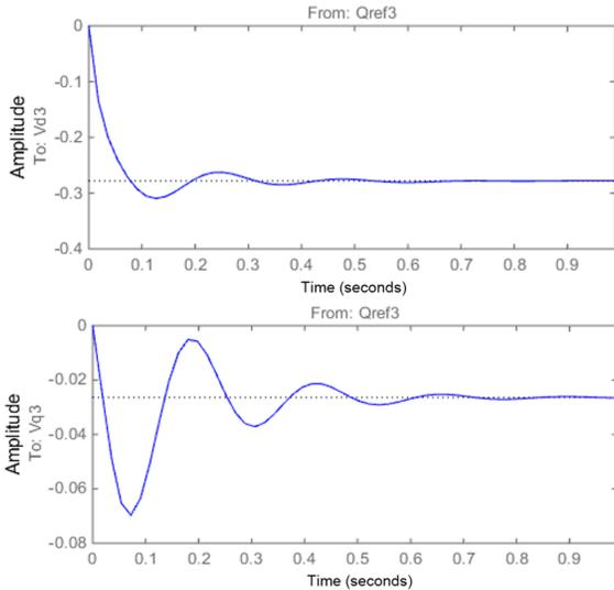
Figure 12. Response of voltage  $V_{dq3}$  from  $Q_{ref3}$
