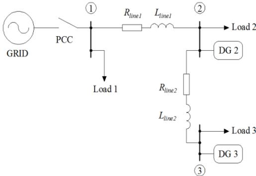
Figure 9. Microgrid in case study
