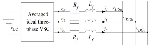
Figure 3. The circuit diagram of VSI
