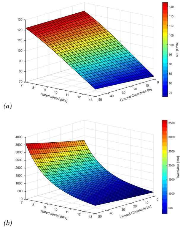
**Figure 9.** Impact of rated speed and ground clearance on (a) AEP and (b) tower mass
