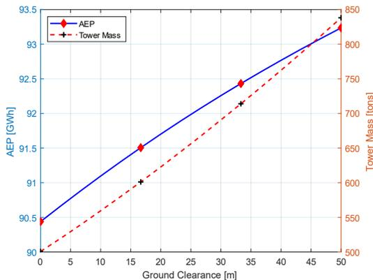
**Figure 8.** Impact of GC on AEP and tower mass
