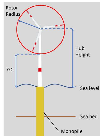
**Figure 1.** Ground clearance concept for offshore turbine
