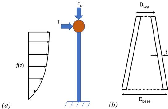
Figure 3. (a) Tower loads model, (b) Tower vertical cross section
