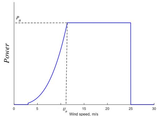
**Figure 2.** Power curve of wind turbine
