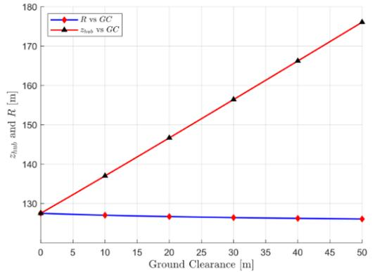
Figure 6. Effect of increasing ground clearance to rotor radius and hub height
