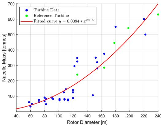
Figure 5. Nacelle mass fitting
