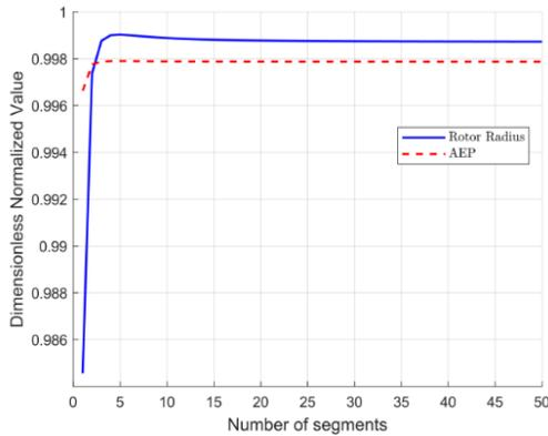
**Figure 7.** AEP and  $R$  vs. Number of segments (Normalized to base values: 127 meters for  $R$  and 91,600 MWh for AEP)
