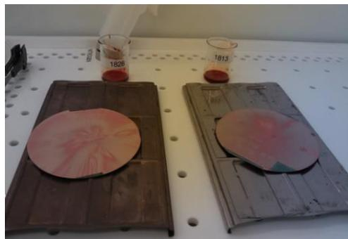
Figure 18. Wafers after coating photoresist (wafer 1 on the right, wafer 2 on the left)
