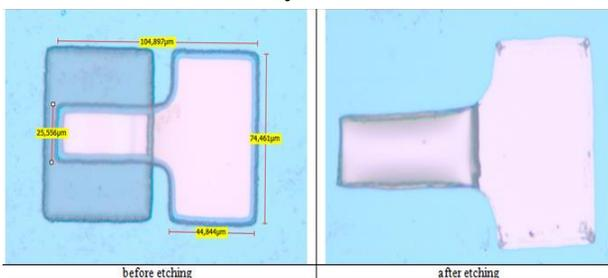
**Figure 27.** Before and after photoresist etching for wafer2
