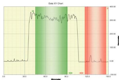
Figure 17. Thickness of Cu layer measured by profilometer
