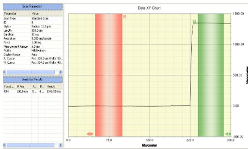
Figure 20. Thickness of photoresist of wafer 2
