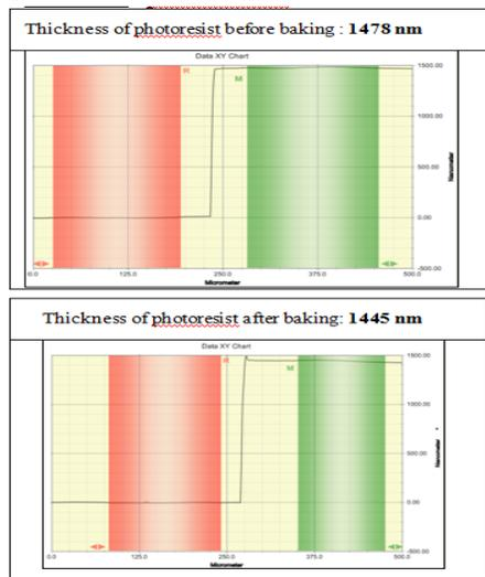
Figure 14. Thickness of photoresist of wafer 1
