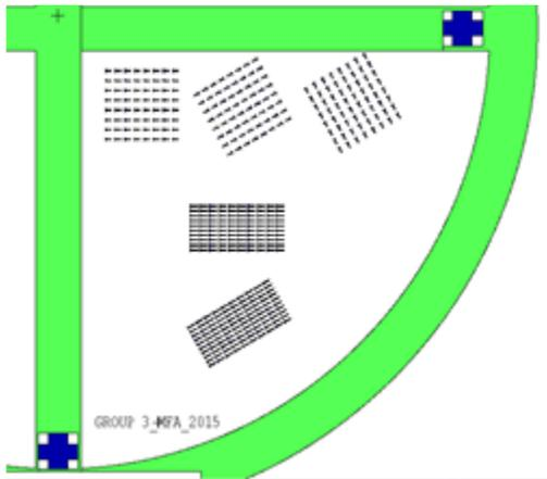
Figure 3. Mask design in L-edit software
