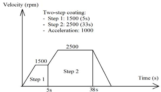
a) Velocity diagram for photoresist S1813
