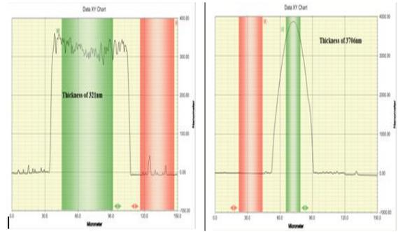
**Figure 28.** Support thickness of cooper after 30min dry etching
