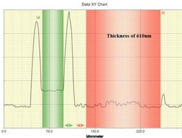
**Figure 26.** Thickness of support after etch
