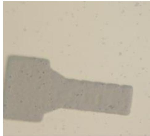
Figure 5. Mask design to reduce residual stress under microscope
