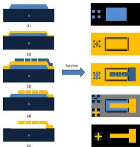
Figure 1. Microfabricated processes of copper cantilever beams
