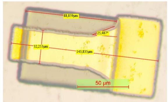
Figure 6. The cooper layer of beam sticks to the substrate due to not good alignment
