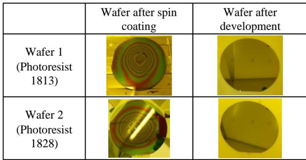
Figure 13. Wafers after spin coating and development
