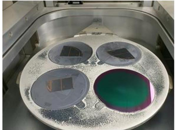
Figure 12. Dry etching chamber
