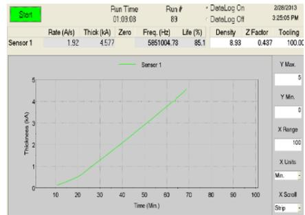
Figure 16. Deposition rate and thickness of copper layer
