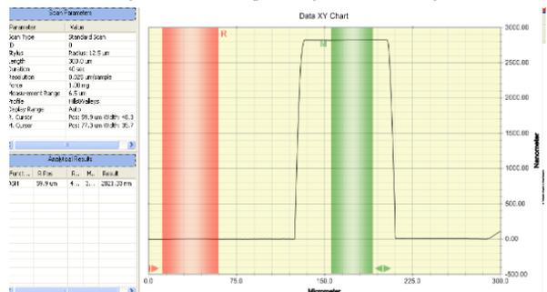
Figure 19. Thickness of photoresist of wafer 1
