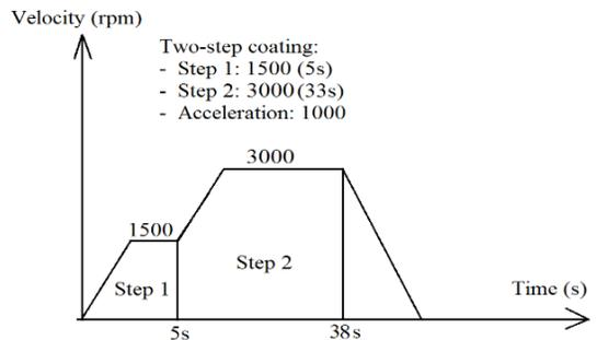
b) Velocity diagram for photoresist S1828
