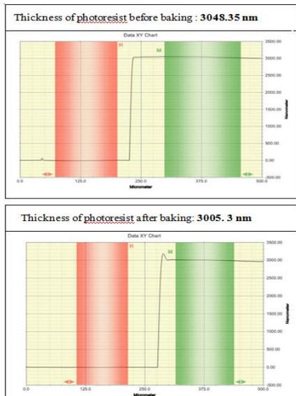
Figure 15. Thickness of photoresist of wafer 2
