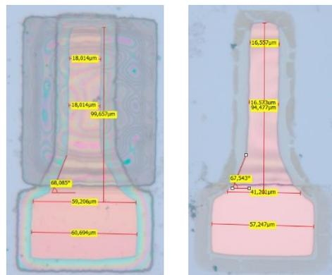
Figure 25. Before and after photoresist etching for wafer1
