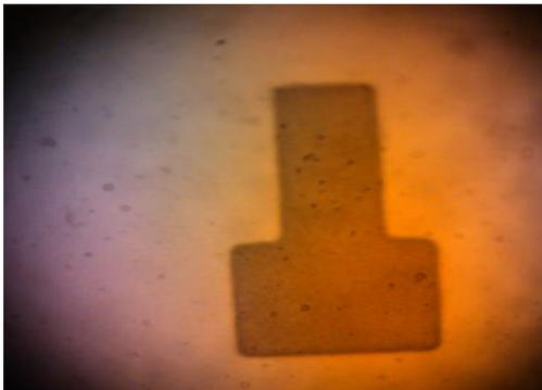
Figure 4. Mask design of normal beam under TEM microscope
