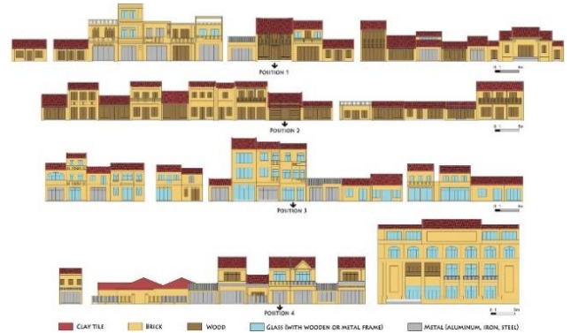
Figure 6. Statistics of materials used in the 100 meters street façade around four measuring positions
