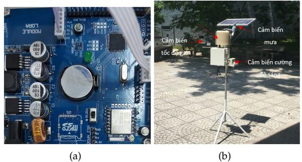
Fig. 10: The sensor station: (a) The main circuit board; (b) Installation on a rack.
