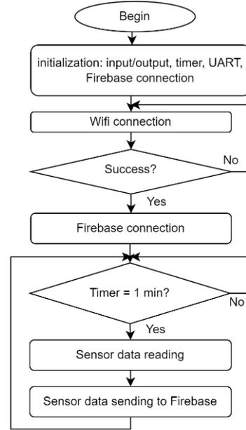
Fig. 3: The algorithm diagram for the sensor station.
