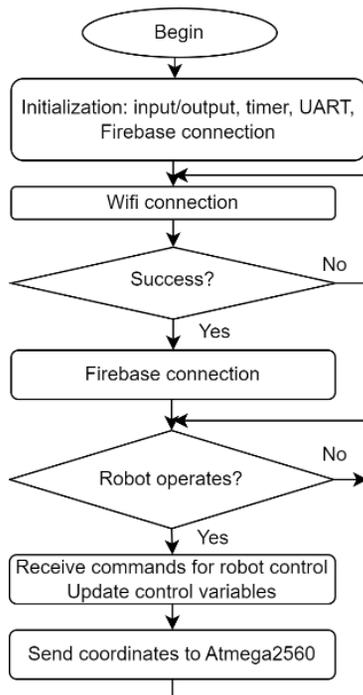
Fig. 8: The algorithm diagram for receiving and sending data to Firebase.
