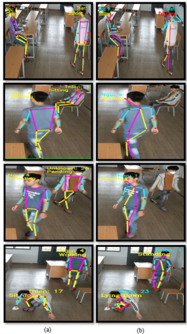
Fig. 7: The qualitative result of (a) YOLOv7-Pose + ST-GCN and (b) YOLOv3 + AlphaPose + ST-GCN.
