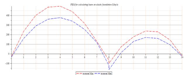
Figure 12. Interval moment graph in FEM.BEF
