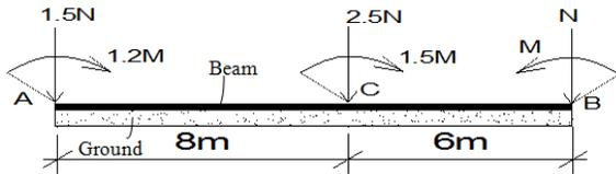
Figure 5. Structure diagram of foundation beam under load
