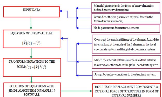
Figure 4. Block diagram of structural analysis steps
