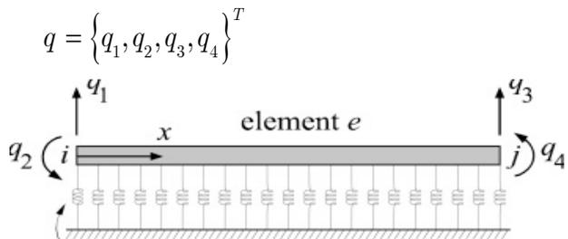
Figure 3. Element diagram of beam on elastic foundation
