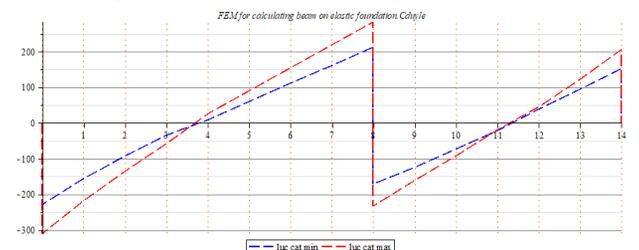
Figure 13. Interval shear graph in FEM.BEF
