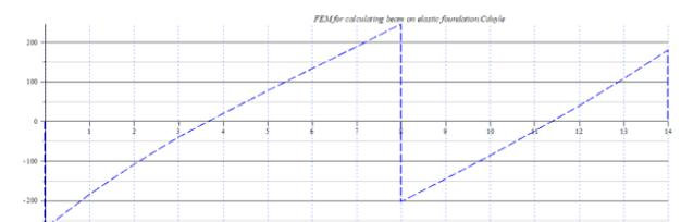
Figure 10. Shear graph in FEM.BEF
