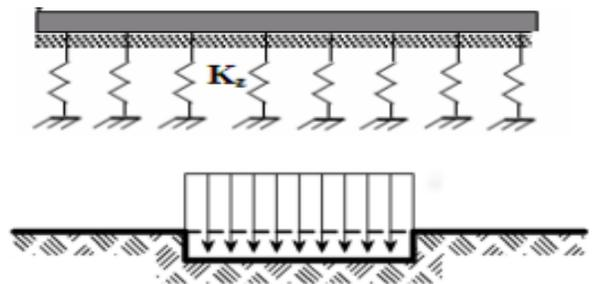
**Figure 1.** Beam on elastic foundation – Winkler ground model
