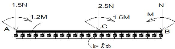
Figure 6. Calculation model of beams on elastic foundation
