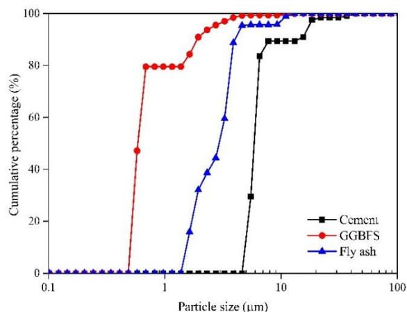
**Figure 1.** The gradation curves of cement, fly ash, and GGBFS particles
