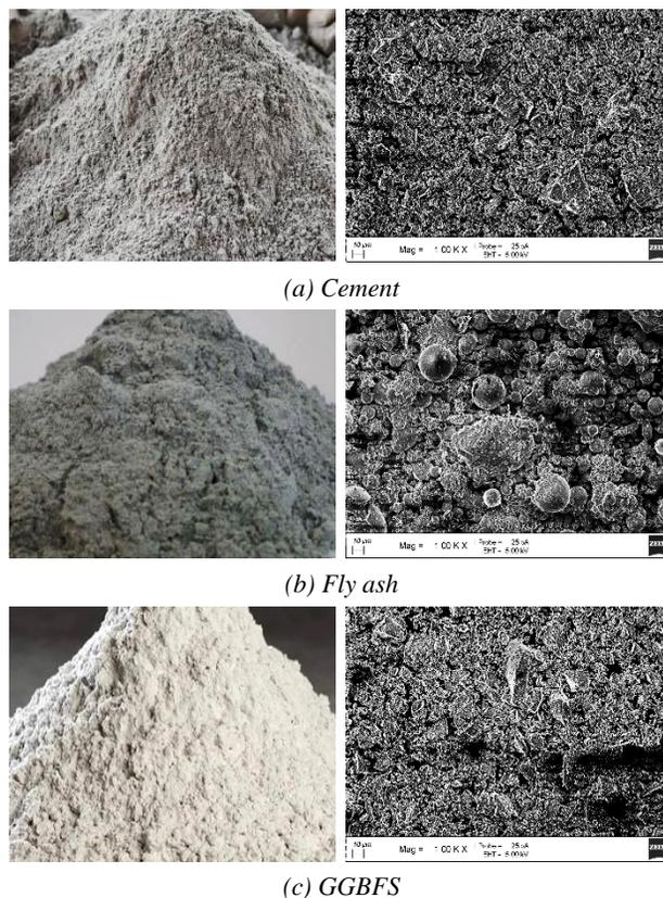
**Figure 2.** The natural appearance of binder materials and their SEM micrographs
