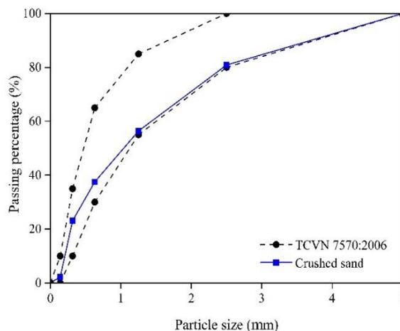
**Figure 3.** The particle size distribution of crushed sand
