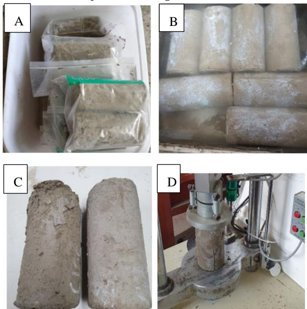
Figure 2. (a) separate specimens before curing, (b) submerged samples, (c) damaged specimens after curing, (d) UCS test
