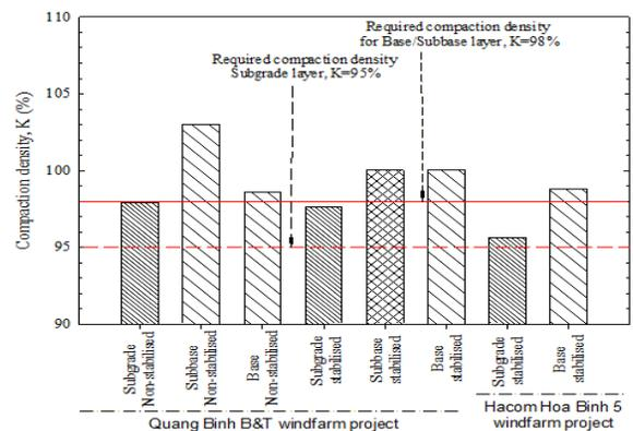
**Figure 11.** Compaction density results of trial section in Quang Binh B&T windfarm and Hacom Hoa Binh 5 Projects
