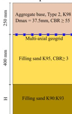
Figure 8. Stabilised structure for the unpaved road in Hacom Hoa Binh 5 windfarm project
