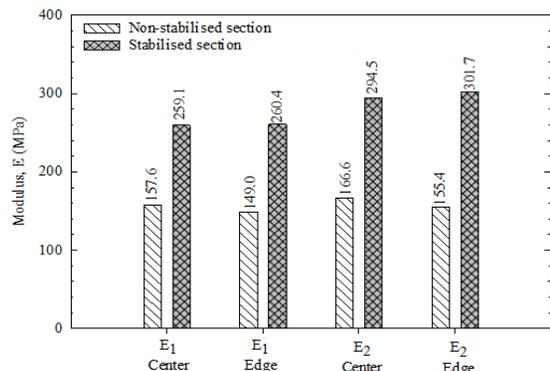
**Figure 12.** Elastic Modulus of Non-stabilised section with stabilised section at difference tested location in Quang Binh B&T windfarm project
