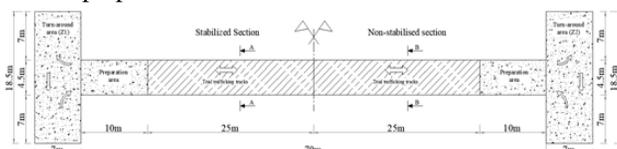
Figure 5. Detail plan view of trial construction for access road
