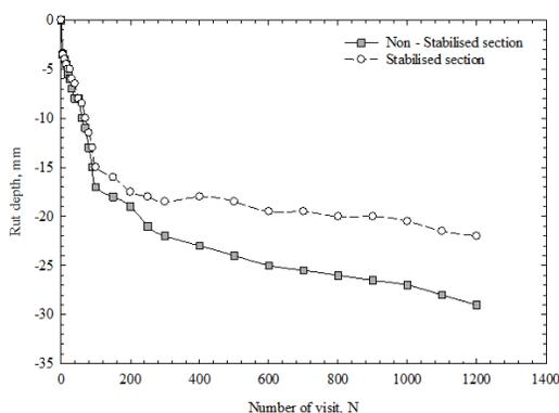
**Figure 14.** Trafficking test results for non-stabilised and stabilised section in Quang Binh B&T windfarm project
