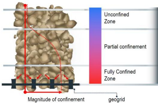
Figure 2. Confinement zones in MSL structure [10]
