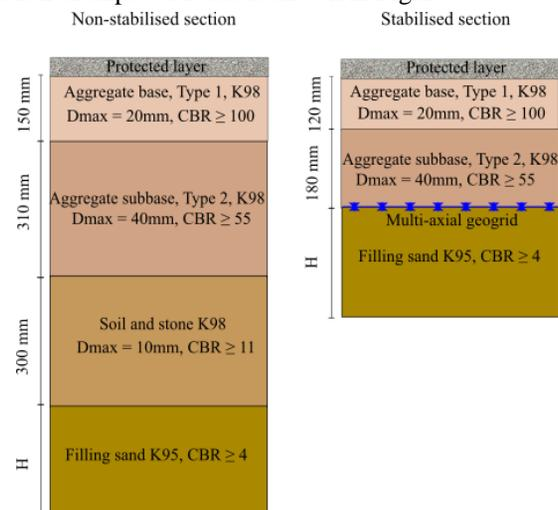
Figure 4. Non-stabilised and stabilised structure for the unpaved road
