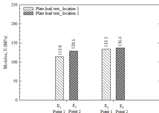
**Figure 13.** Elastic Modulus of stabilised section at different tested location in Hacom Hoa Binh 5 windfarm project
