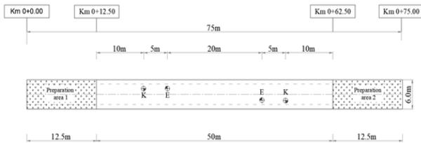
**Figure 9.** Plan view of trial construction in Hacom Hoa Binh 5 windfarm project
