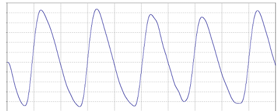
Figure 9. The output waveform of Sallen-key high pass filter
