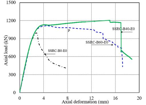
Figure 7. Axial load-deformation relationship of the concentrically compressed columns
