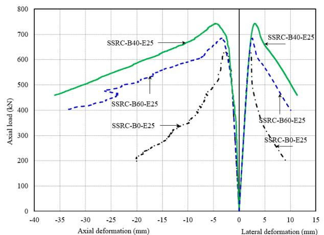
**Figure 9.** Axial load-deformation-lateral deformation relationship of the 15 mm eccentrically compressed columns (mm)
