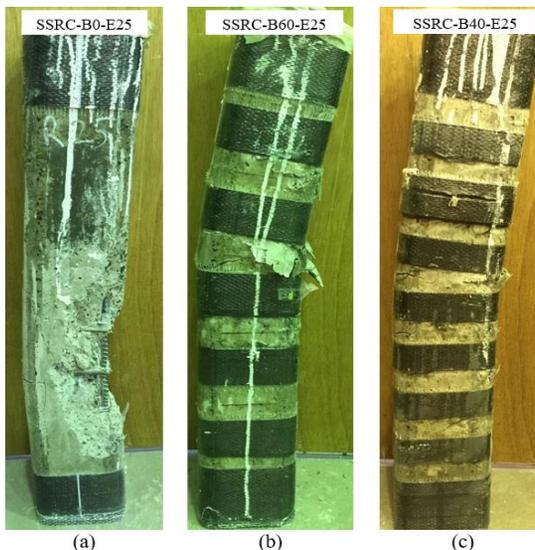
**Figure 5.** Failure modes of specimens tested under 25 mm eccentric compression: (a) Column SSRC-B0-E25, (b) Column SSRC-B60-E25, and (c) Column SSRC-B40-E25
