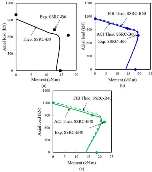
**Figure 12.** Comparison between the experimental and theoretical P-M diagrams: (a) Group SSRC-B0, (b) Group SSRC-B60, and (c) Group SSRC-B40
