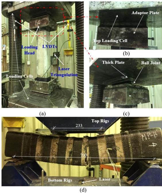
**Figure 2.** Loading system and instruments: (a) test setup of the EC-SSRC column, (b) loading head system for concentrically loaded specimens, (c) loading head system for eccentrically compressed columns, and (d) test setup of the column under pure bending
