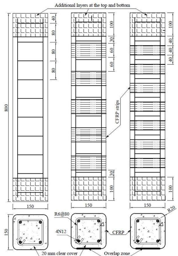
**Figure 1.** Details of the reinforcement and geometry of SSRC columns (mm): (1) Group SSRC-B0; (2) Group SSRC-B40; (3) Group SSRC-B60
