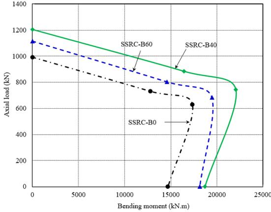
Figure 11. Experimental axial-flexural interaction diagrams
