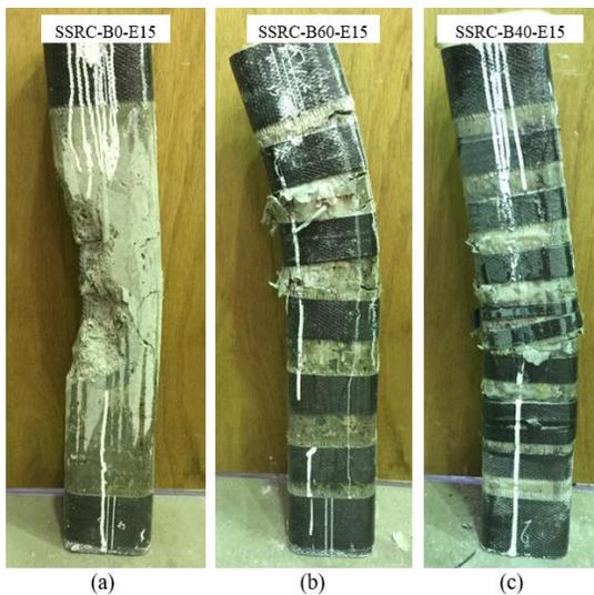
**Figure 4.** Failure modes of columns tested under 15 mm eccentric compression: (a) Column SSRC-B0-E15, (b) Column SSRC-B60-E15, and (c) Column SSRC-B40-E15
