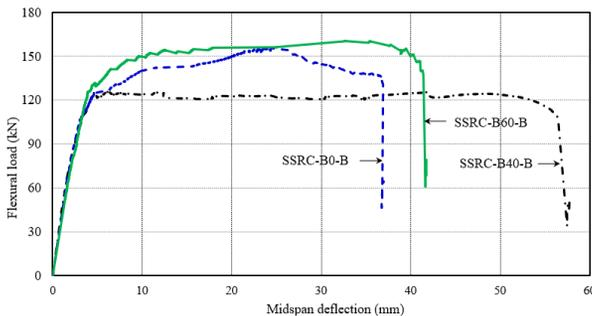
**Figure 10.** Load-midspan deflection relationship of columns under four-point bending (mm)
