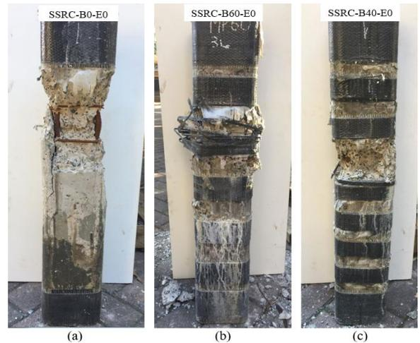
**Figure 3.** Failure modes of SSRC columns under axial compression: (a) Column SSRC-B0-E0, (b) Column SSRC-B60-E0, and (c) SSRC-B40-E0
