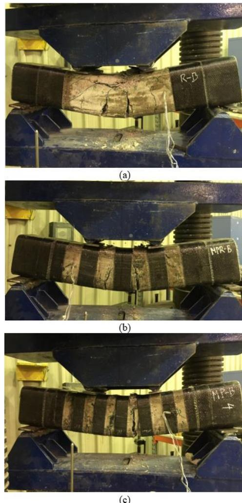
**Figure 6.** Failure modes of columns tested under four-point bending: (a) Column SSRC-B0-B, (b) Column SSRC-B60-B, and (c) Column SSRC-B40-B
