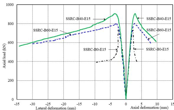
**Figure 8.** Axial load-deformation-lateral deformation relationship of the 15 mm eccentrically compressed columns (mm)
