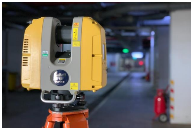
Figure 7. Orientation using a total station prism and scan with the 3D Scanner – GLS2000
