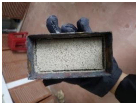
Figure 3. Sample formed by pouring method after firing
