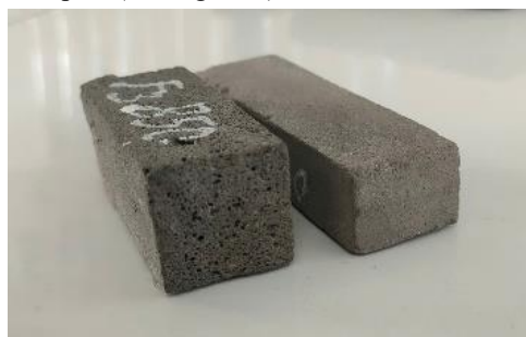
Figure 4. Sample formed by semi-dry pressing method after firing
