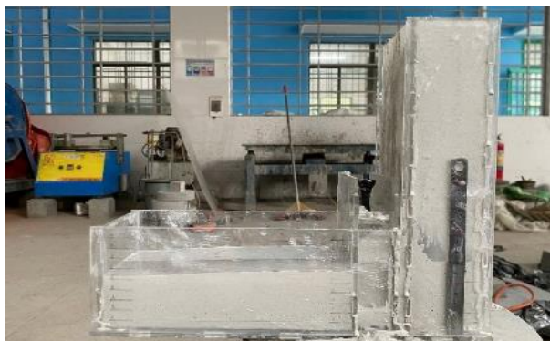
Figure 3. L-box test apparatus
