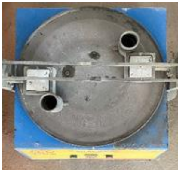
Figure 2. Abrasion testing equipment according to TCVN 3114:2022
