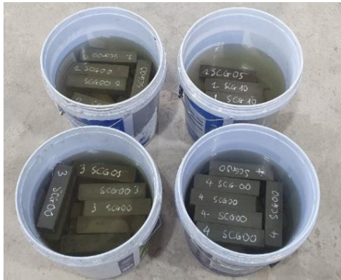
Figure 4. Mortar samples immersed in different solutions
